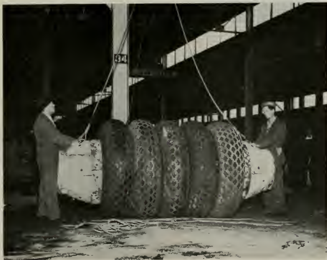
Ship's dockside fender for use at Buenos Aires with Inventor Vic Knudsen standing at left.
